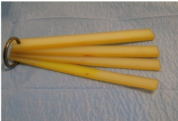
Fig. 1 The tool for measuring condylar lift-off consists of four spatulas made of polyethylene of increasing thickness
